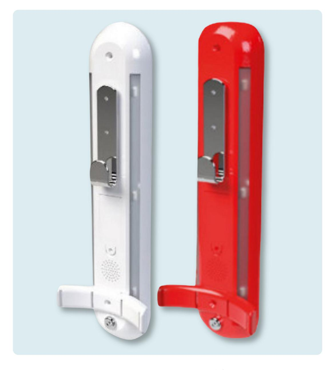
The FireShield X-Alert is an innovative extinguisher mount that combines a wide-base backboard for stable weight distribution with a built-in anti-theft alarm. It features 12 ultra-bright SMD LEDs and a loud 100dB siren, triggered when the extinguisher is removed.
